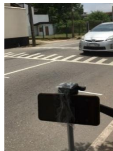
Figure 6: Smartphone placed on a tripod to obtain the noise level
