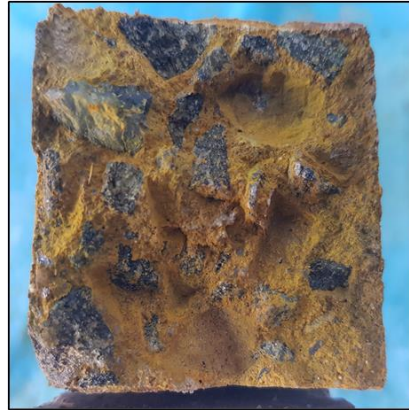
Figure 7. Control/Water specimen treated with Sodium Cobaltinitrite after applying KOH drops on the surface
