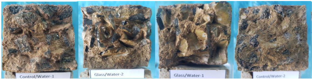
Figure 2. Concrete specimens are cured in water (Batch 2).
