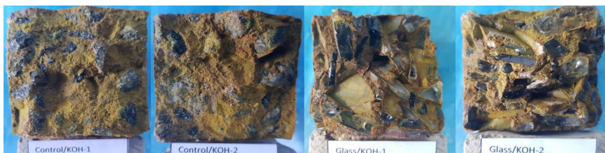
Figure 6. Concrete specimens cured in 1M KOH (Batch 2)
