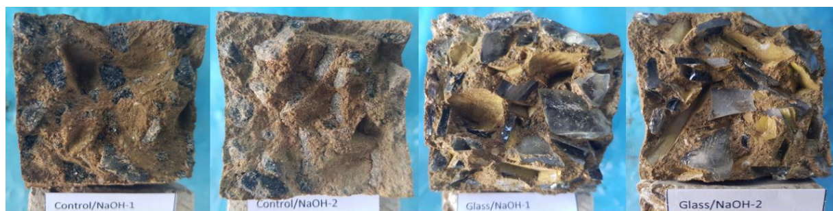
Figure 4. Concrete specimens cured in 1M NaOH (Batch 2)
