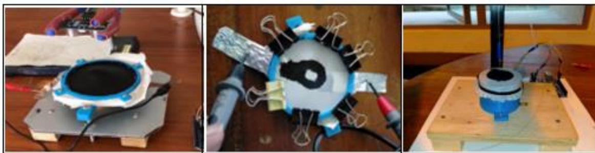
Figure. 01. Designs proposed for the clapping of the dielectric polymer film (from left to right) (a) Design I (nut/bolt) (b) Design II (paper clips) (c) Design III (cable-tie)
